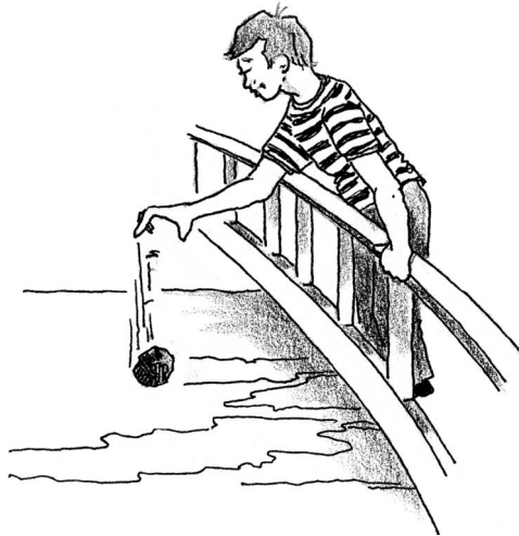
FIGURE 2.6 After a time t , the instantaneous velocity of the stone that the boy drops from the bridge is v = gt .
