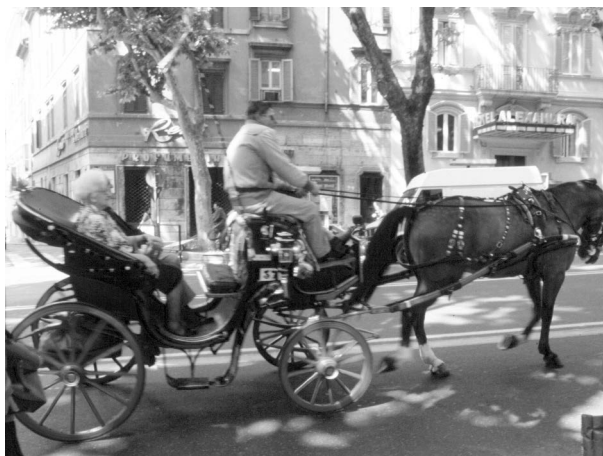
FIGURE 4.3 The force exerted by the horse is in the same direction as that of the resultant motion. In this case, the work done by the horse is equal to the product of the magnitude of the force and the distance traveled.
