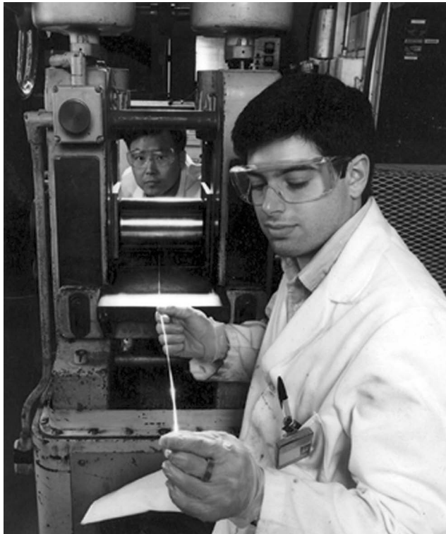
FIGURE 13.18 Superconducting wire developed at Argonne's National Laboratory. (Courtesy of Argonne National Laboratory.)
