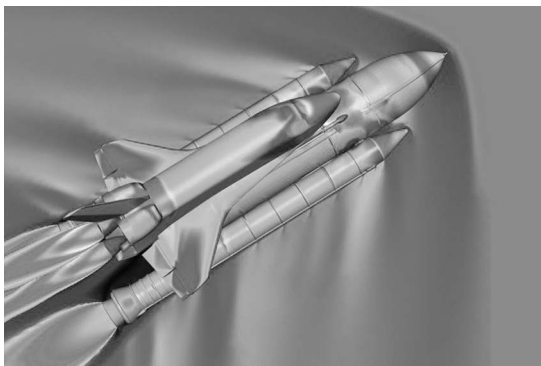
FIGURE 16.14 Shock wave formed by a source of sound moving at supersonic speeds. (Courtesy of R. J. Gomez, NASA Johnson Space Center.)
