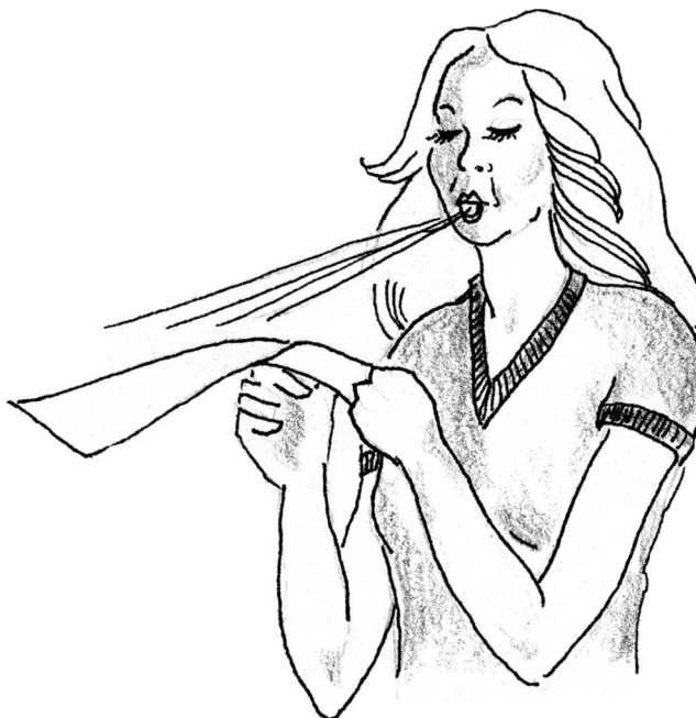
FIGURE 9.19 The pressure from the bottom, where the air is still, is larger than the pressure from above, where the air is moving as you blow. This net pressure upward lifts the paper.
