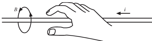
FIGURE 14.5 The right-hand rule to determine the direction of the magnetic field around a current-carrying wire. If the right thumb points in the direction of the current, the curled fingers indicate the direction of the magnetic field.
