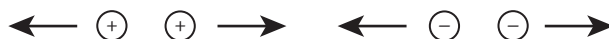
FIGURE 25.2 Changing the sign of all the individual charges produces no effect on the forces between them.
