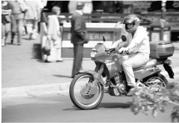
FIGURE 10.2 Friction between the wheels and the brake pads makes the wheels hot. The tires also get warm after the motorcycle has been driven due to friction with the pavement.
