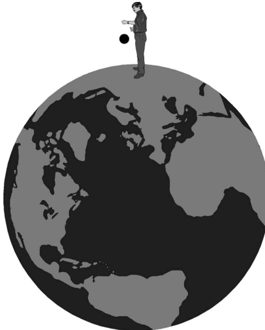
FIGURE 3.11 The earth pulls on the falling ball with a force that we call the ball’s weight. The ball pulls on the earth with an equal and opposite force.
